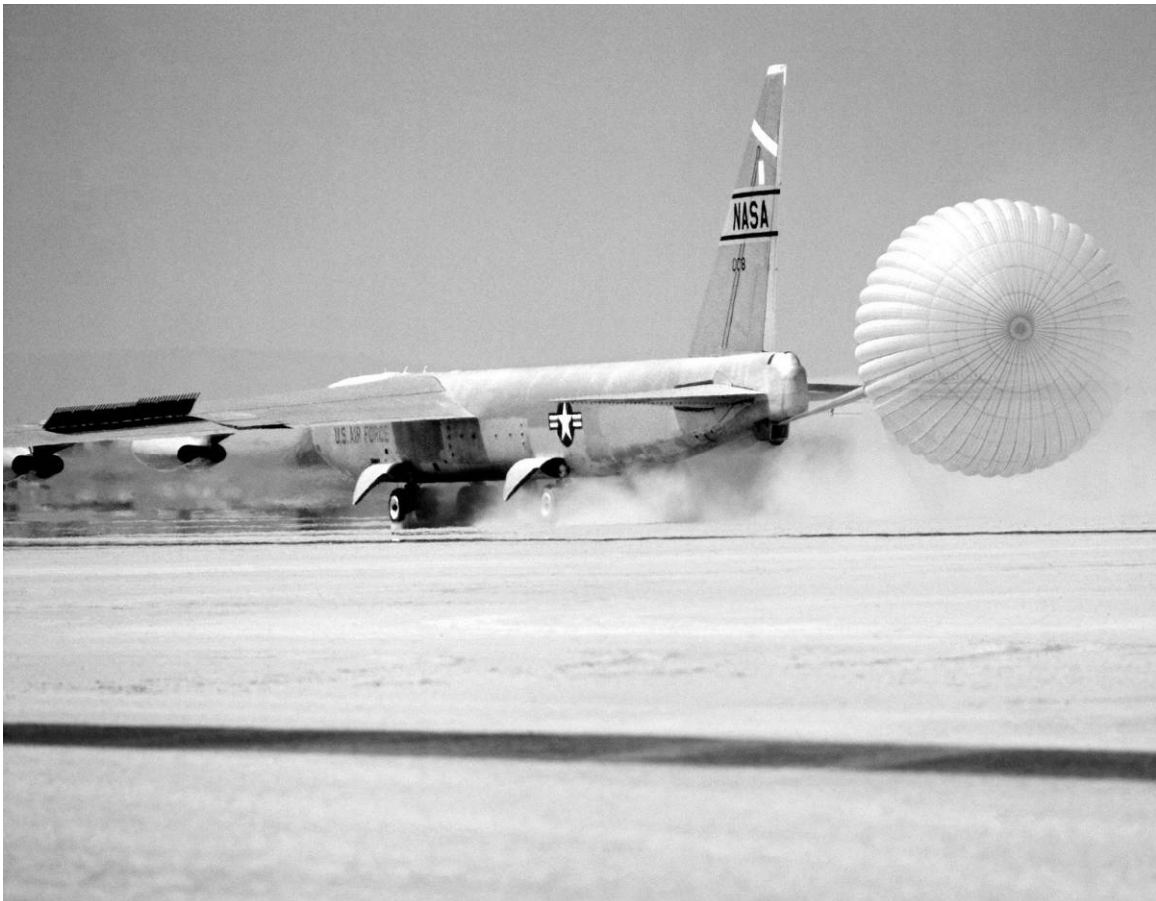
Figure No. A-33. A B-52 testing the Developmental Space Shuttle drag chute, 1990. Source: NASA Dryden Flight Research Center, EC90-225-30, accessed May 2012, at http://www.dfrn.nasa.gov/gallery/photo/B-52/Small/EC90-225-30.jpg .
